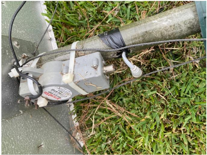
There's a legal limit 4:1 balun (also from ebay) that's used for impedance matching the multiband dipole elements to the 50-ohm coax at the feed point. I will not delve into the underlying dipole design in any detail, as there are plenty of off-the-shelf and well-designed multi-band wire dipoles to choose from today.
