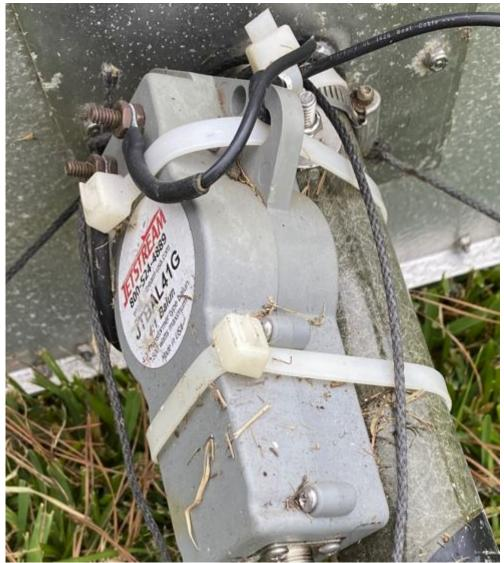
The above closeup shows the top of the fiberglass mast mounted to the bottom of the birdhouse using a stainless steel bolt with an aircraft nut. There's also a hose clamp around that area, which acts as a backstop for the guy lines. The antenna elements are looped through the strong plastic balun, which is strapped to the mast using very strong white tie wraps. This is all the ugliness of the antenna that is hidden from plain sight using the upside-down irrigation value cover.
